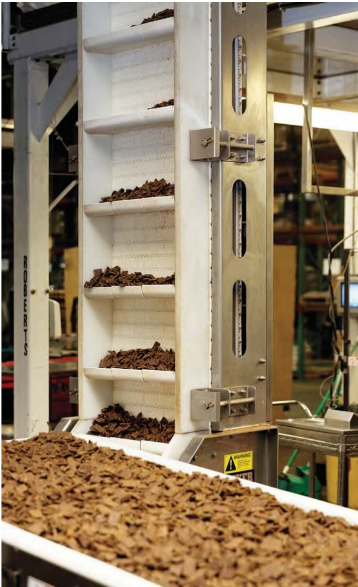
Top: Quality manager Maria Fessler tests samples for moisture. Bottom: A bucket conveyor carries product to packaging.
